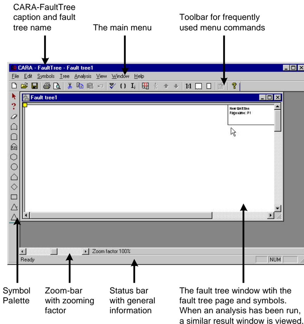
The procedure to create a new fault tree, enter some data and run an analysis is described in detail below:
